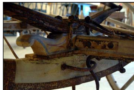
To right: Vertical "King Bolt" or "King Pin" holds axle to running gear. Axle swivels on steel plates. Safety hook is in case pin falls out! Note the curved carving on the upper plate. The mark of a violin maker?
