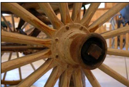
Above: Sarven style hubs to hold wheel spokes to central hub.
